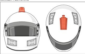
Before installing the Forced Air insert, remove the protective cover from the back side of the Forced Air insert exposing the adhesive material that will seal the Forced Air insert to the helmet shell. Once installed press firmly around the edges of the Forced Air insert to assure proper adhesion.
