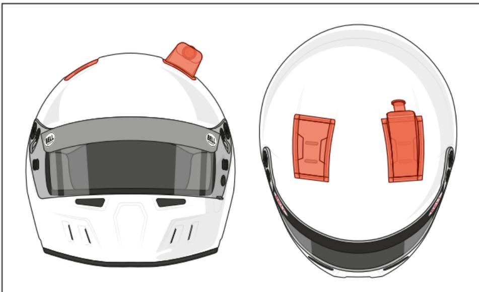
Before installing the Forced Air insert and the Cover Plate, remove the protective cover from the back side of the Forced Air insert and the Cover Plate exposing the adhesive material that will seal the Forced Air insert and the Cover Plate to the helmet shell. Once installed press firmly around the edges of the Forced Air insert and the Cover Plate to assure proper adhesion.
