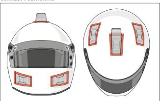
Place the Forced Air and Cover Plate Seals on top of the Forced Air inserts or on top of the Cover Plates to ensure a perfect seal and prevent air escaping or entering (illustration 01).
