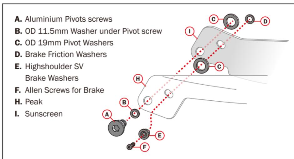
3. Remove the peak and the old sunscreen and if necessary replace the pivot and friction washers. New washers have a self-adhesive side to be applied on the helmet shell.
