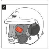
**2.** Attach the foam spacer to the interior of the helmet with the male velcro.
