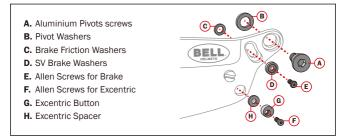
3. Remove the old shield and if necessary replace the pivot and friction washers. New washers have a self-adhesive side to be applied on the helmet shell.
