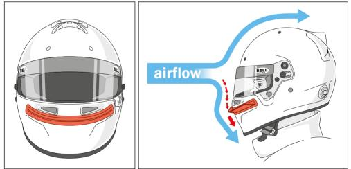
Center the Chin Bar Gurney just below the chin bar vents and mark points of reference. Remove the protection tape from the adhesive and place the Chin Bar Gurney on the helmet starting from the middle and let it fall in position (avoid tension). Press firmly on the edges for good adherence.
