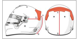
Take points of reference by measuring the position of the spoiler as shown on the diagrams and according to your helmet size. (See chart below)
