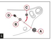
To stack tear-offs: Use a coin or screwdriver to turn the adjustable tear-off posts so that the widest part of the posts are towards the center of the face shield.
